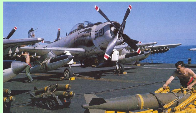
Loading bombs on outer wing racks usually required spreading the wings
