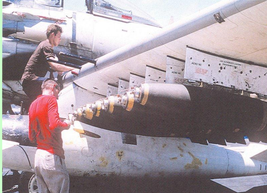
Red-shirt arms 250-lb bombs on the flight deck. Two 20mm cannon are above the Red-Shirt and cockpit bolt-on armor is behind the Brown-Shirt.
