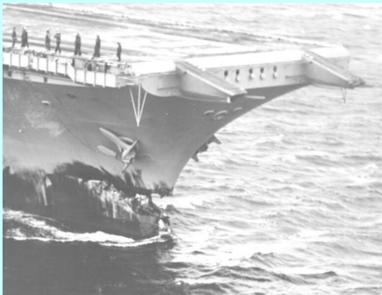
USS RANGER damage after 5 April collision with Liberian tanker FORTUNE near the eastern approaches to the Straits of Malacca.
